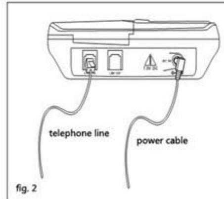
2. Connect the telephone line and power cable to their corresponding connectors at the back of the base station marked **LINE IN** and **DC IN**. (see fig.2)
